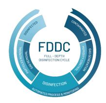
The biological disinfection is done by using a mixture of atomized water and ozone created from the surrounding ambient air. No other consumable is added to the process. The gaseous treatment reaches pathogens everywhere without any shadow areas. Because of this unique process, even the antibiotic resistant bacteria such as MRSA and VRE will not resist this disinfection.
