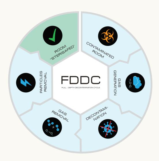
The Full-Depth Decontamination Cycle (FDDC) technology provides a process to decontaminate air and surfaces from all harmful pathogens, such as viruses, bacteria and even the so-called superbugs, the antibiotic resistant bacteria.
